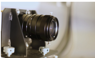
REMOVING SUBTLEST COLOR AND SHAPE DEFECTS Double-sided RGB cameras combined with high intensity, focused LED lighting
